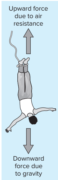
FIGURE 1.1 Forces acting on a free-falling bungee jumper.
